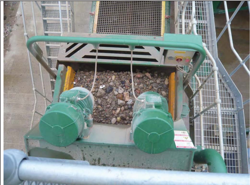
Plate 5 Aerial view of the washing of the aggregate once through the initial crusher.
