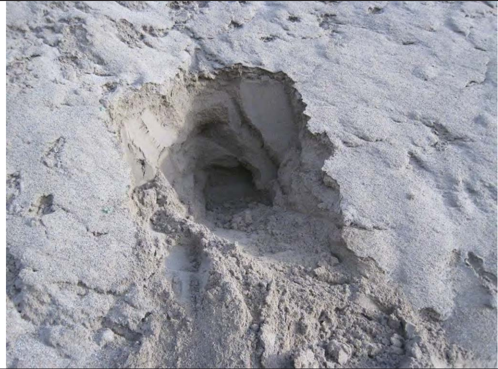
Plate 11 View of a fine RCA stockpile that has been sampled for subsequent laboratory testing.
