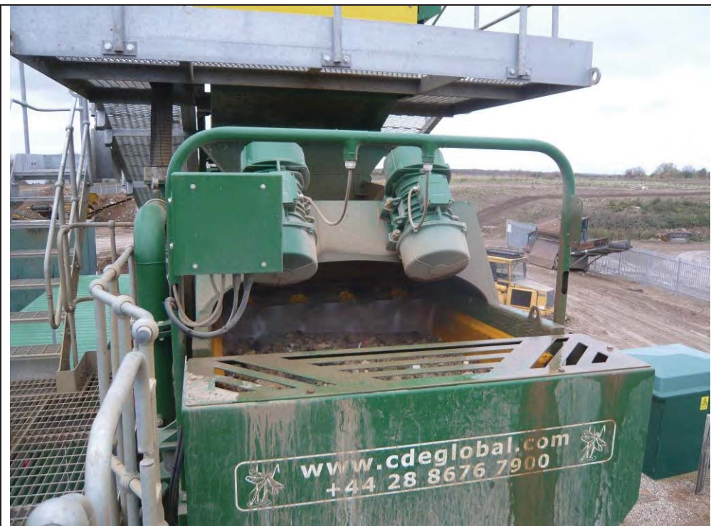
Plate 6 Similar view to Plate 5, showing the washing of the coarse and fine aggregates.
