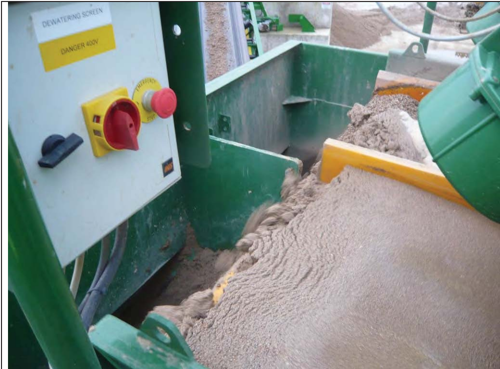
Plate 7 General view of the dewatering screen of the fine RCA.
