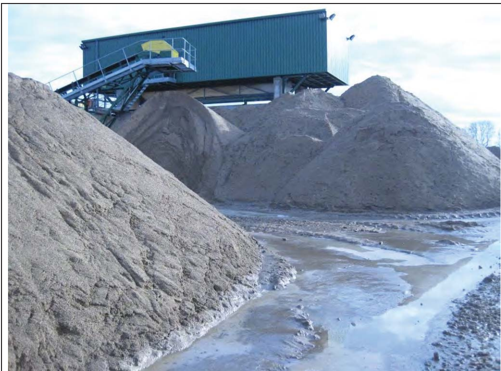
Plate 10 General view of the fine RCA stockpiles.
