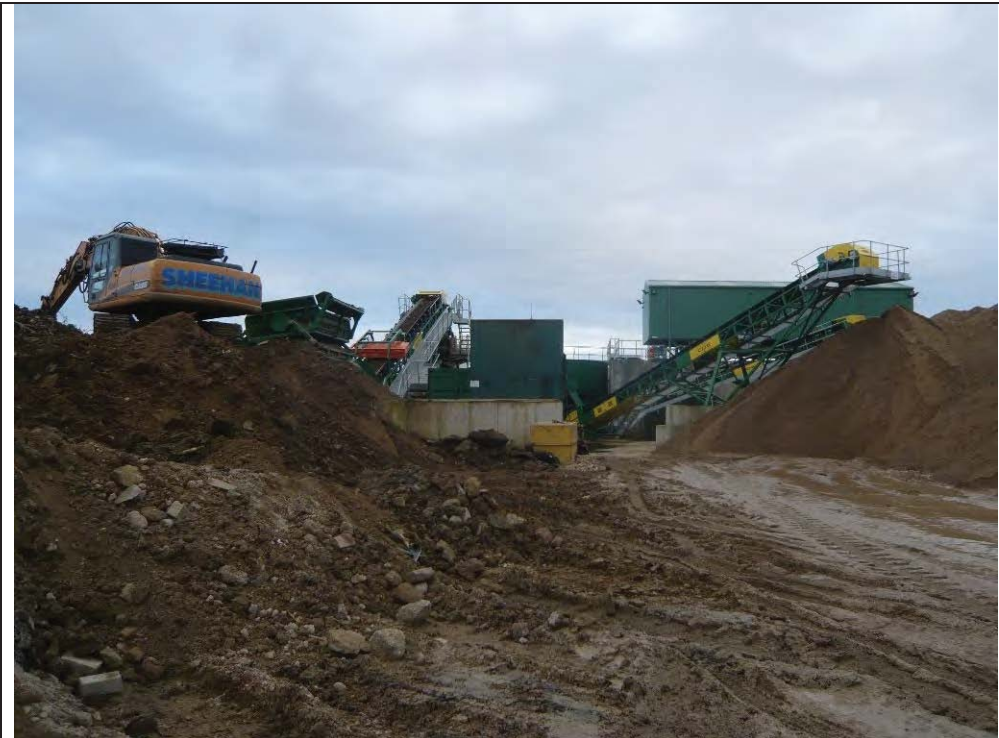
Plate 3 General view of the plant, showing the loading of the material on the left-hand side of the photomicrograph and the processed fine RCA on the right-hand side.
