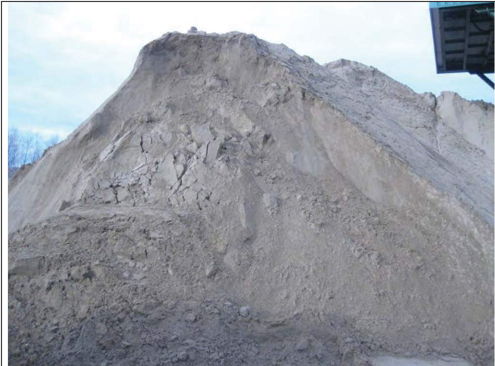
Plate 9 General view of a fine RCA stockpile.
